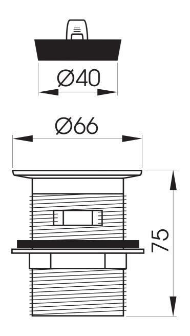
TW-171 40mm Waste with Overflow and Rubber Plug
